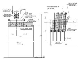
\* The sheet folded area occupies about 1/4~1/5 of the total opening width. Weight: Approx.5kg per meter (not including the weight of the sheet)
