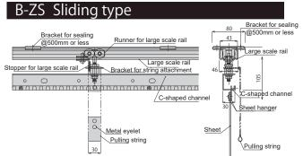
Weight : Approx.2.8kg per meter (not including the weight of the sheet)
