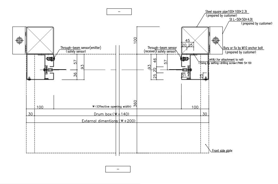
\*\*Construction of bases for installation should be discussed at each site according to the site conditions.
