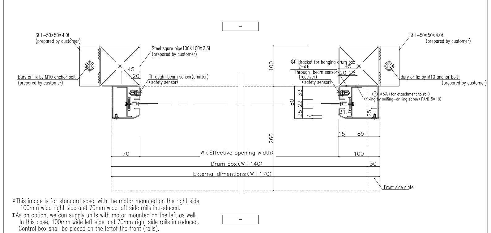
\*Construction of bases for installation should be discussed at each site according to the site conditions.
