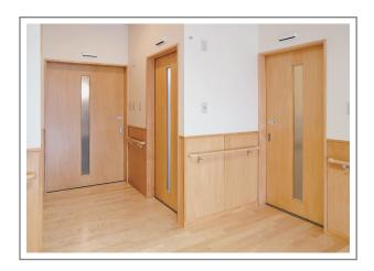
The door operates quietly, smoothly and less friction is generated with the same driving principle as an environmentally friendly linear motor car. Linear motor type sliding doors are highly suitable for places where dust and noise are unfavorable, such as hospitals, laboratories, offices, food factories, etc.
