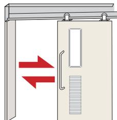
It is possible to deal with a sloped rail system in which the rail on the upper portion of the door is sloped downward so that the door closes due to its own weight. It is a thin and lightweight type with a thickness of 28 mm.
